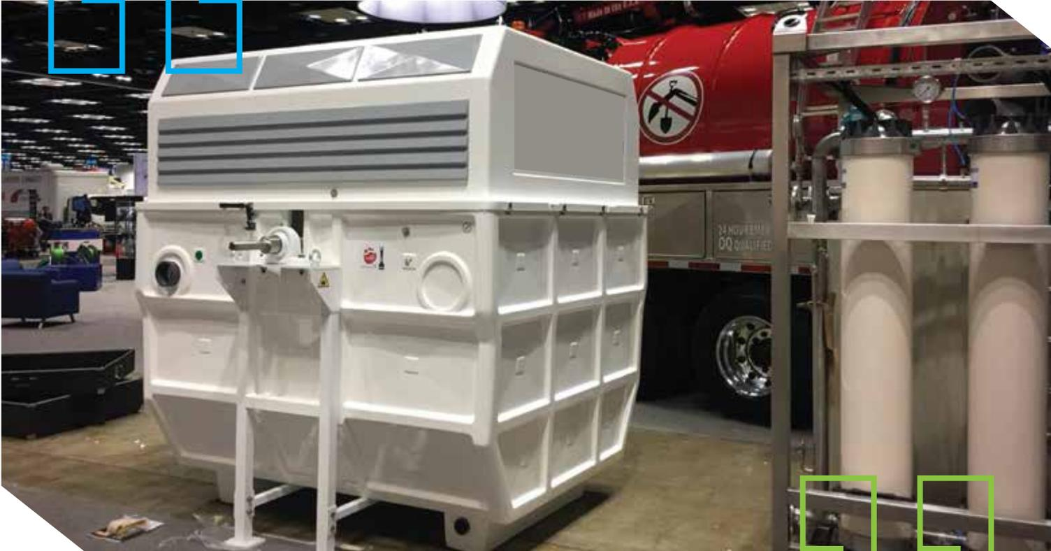
RBC systems are highly stable and efficient solutions for wastewater treatment. These systems are usually operated as post treatment for activated sludge processes in conventional domestic black or gray water treatment, or as decentralized treatments for small to medium sized residential areas, industries or institutions. RBCs can achieve a high removal from biodegradable organic pollutants as well as high-strength industrial wastewater.
