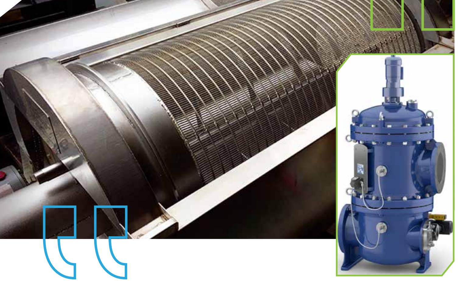
Based on the removal rate required, the particles are filtered through regardless of their structure or density. The removed particles that are accumulated on the filter is vacuumed with 100% backwash efficiency. The backwash process is dependent on the pressure difference. Filtration is continuous during the backwashing process. The filter element can be easily changed based on the required filter sensitivity.
